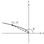
x = x-coordinate of particle's location y = y-coordinate of particle's location  $\theta$  = angle of inclination of line joining the particle to the origin
